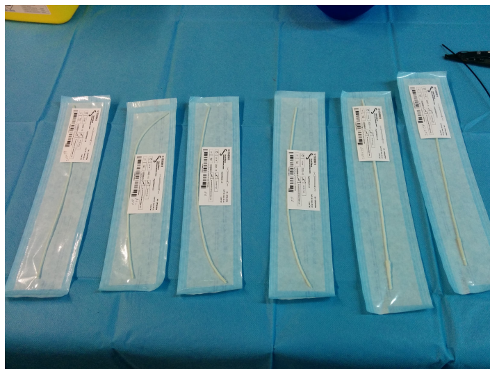
Figure 1 – Biodegradable ureteral stents from natural origin polymers prepared.
