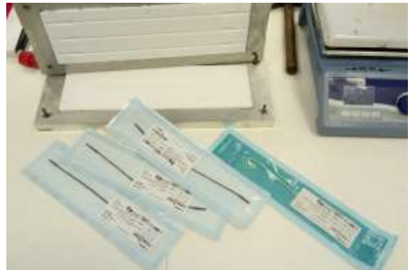
Figure 1 Ureteral stent mould (top) and packaged biodegradable ureteral stents (bottom).
